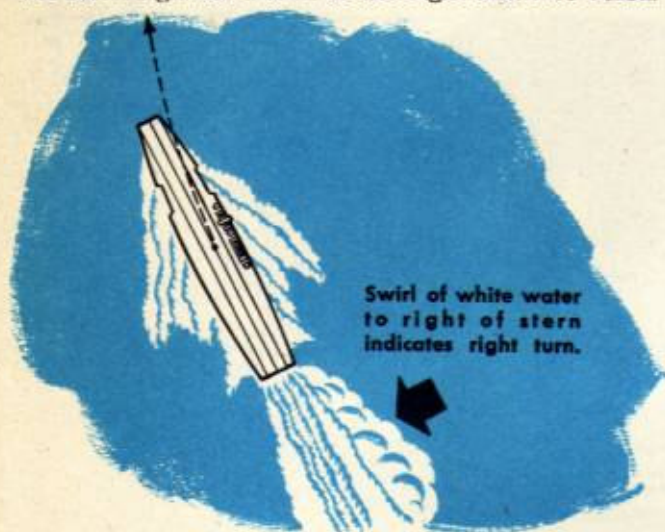
Theoretical aiming point for a turning vessel after obtaining synchronization on its foremast and just prior to release.
