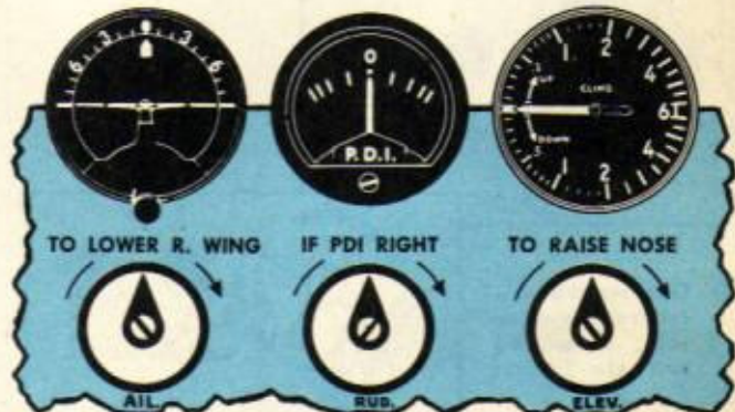
9.-10.-11. Turn aileron, rudder, and elevator switches ON and adjust for straight and level flight.
