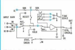
3 Block diagram illustrating flexibility of circuit and patching convenience. Note that • terminals are brought out to patch panel.
