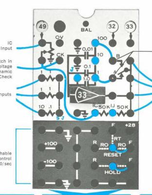
Patchable Time Scales 3 Capacitors (Master Time Scale Controlled by One Switch on Control Panel)
