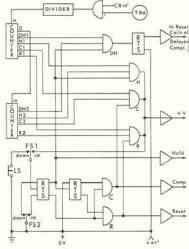
Figure 2. Iterative Operation Logic Control Circuit
