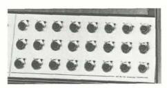
SD 10/20 — Model 3374 Pot Group: The same high-resolution coefficient potentiometers specified for the SD 80 Computer are also included as standard on the SD 10/20. A Model 3374 Pot Group is comprised of 6 coefficient potentiometers. Maximum mounting capacity is four 3374 groups totalling 24 coefficient potentiometers.
