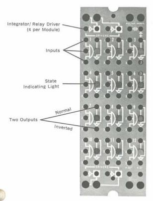
The Model 3327 contains 12 identical AND gates and four relay drivers. Each gate has three input terminals, two output terminals and a state indicating lamp.
